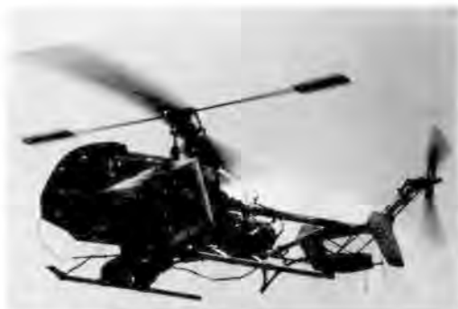
Brian Parkin's radio controlled helicopter carrying an ATV camera and transmitter.
